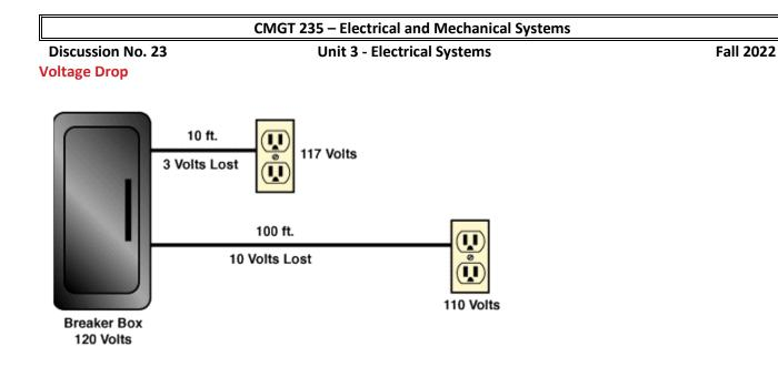
Most building electrical calculations solve for current or voltage drop.
