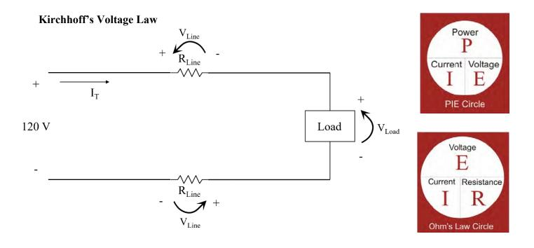
$\Sigma V_{\text{Loop}} = 0$
