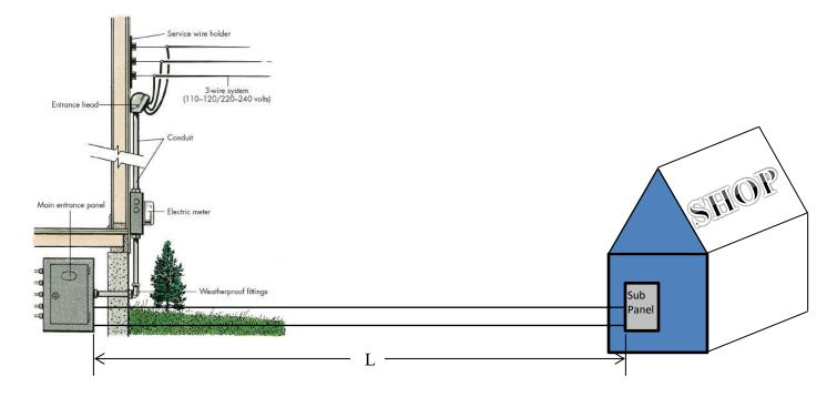
Total connected load for all the lights and equipment in the shop is 15 kW.
